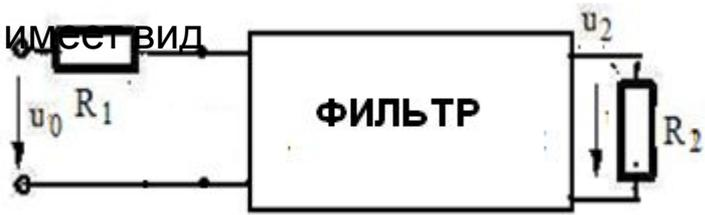
$$H_p(p) = \frac{2U_2(p)}{U_1(p)} \sqrt{\frac{R_1}{R_2}} \quad A_p = -20 \lg |H_p(p)|$$
