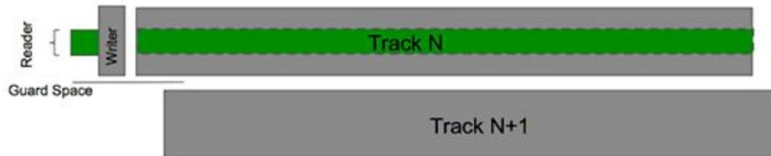
Figure 1. Conventional Track Spacing
