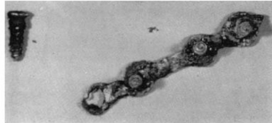
**Fig. 1.** Lane's plate abandoned because of corrosion (1895). (From Bechtol CO, Fergusson AB, Laing PE. *Metals and Engineering in Bone and Joint Surgery*. Williams & Wilkins; Baltimore: 1959. p. 20, with permission)
