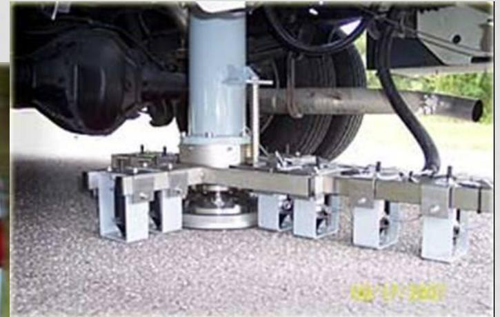
*Dynatest 8000 TMD (Truck Mounted Deflectometer)*
