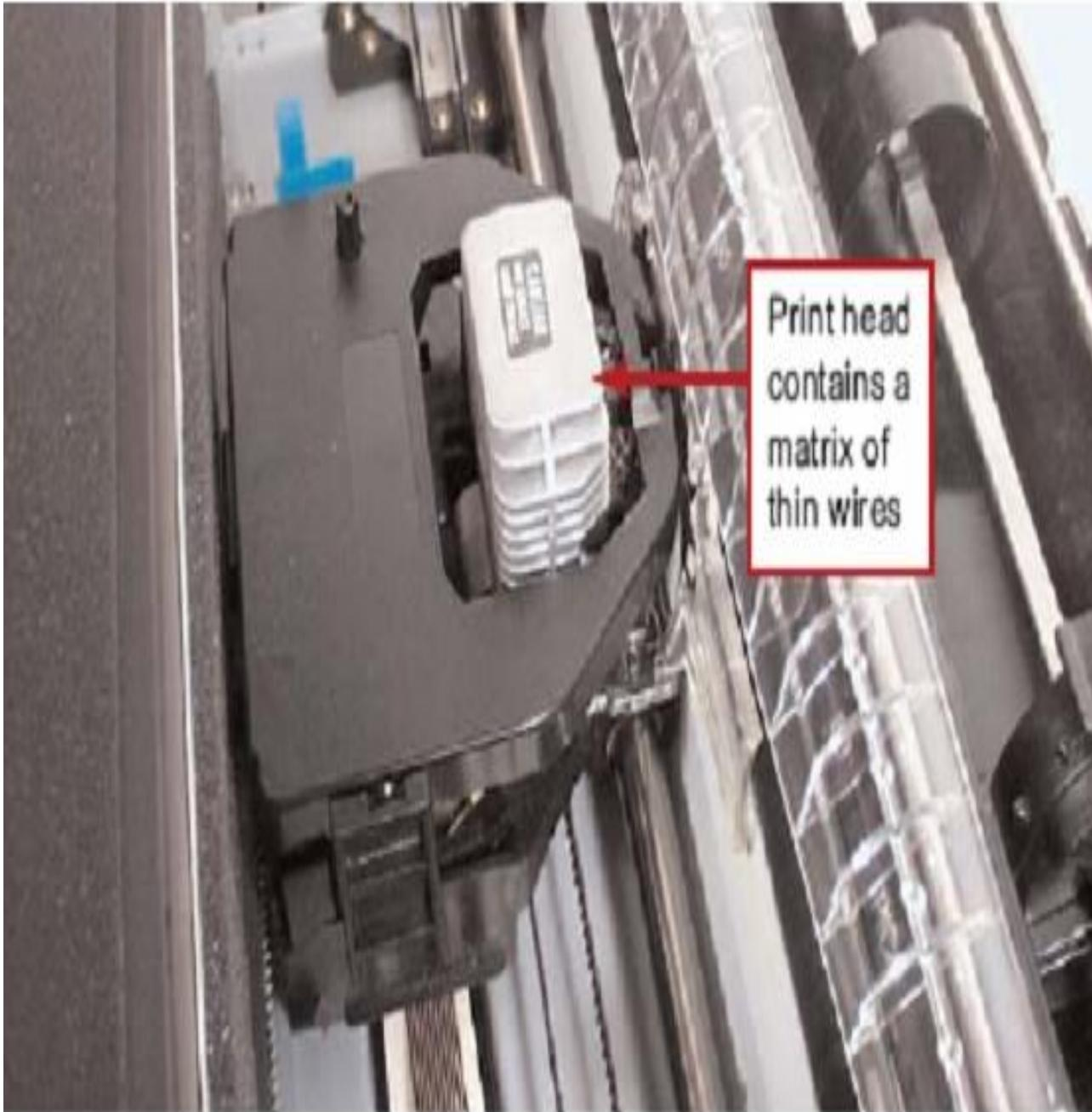
Print head contains a matrix of thin wires
