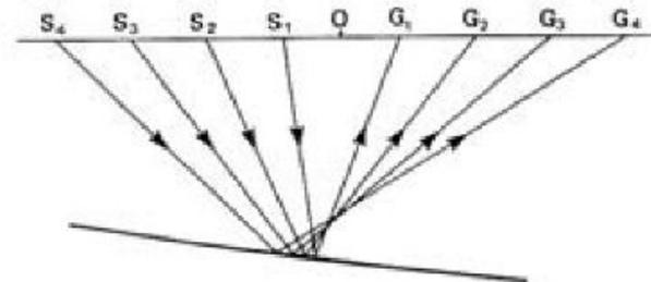
Fig. 4.16 (a) Ray paths of reflections belonging to the common-depth point (CDP) which is located below the shot-geophone common midpoint, O. The arrangement shown gives a six-fold coverage of the subsurface reflection point, R, on a horizontal reflector. (b) For a dipping reflector, the reflection point is not vertically below the shot-geophone midpoint, O.
