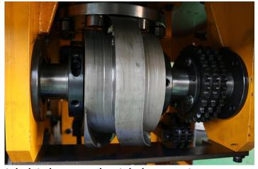
**Gear drive:**This system ensure the machine runs with high speed with low noise, smoothly running and high precision. Instead of chain drive.
