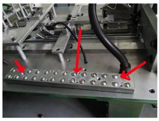
**Bottom paper roller holder:** add the air cylinder at this parts, have control panel. When worker change the roller, just need to adjustment the height of holder, do not need to move the roller up. As a woman, also easy to change the roller.
