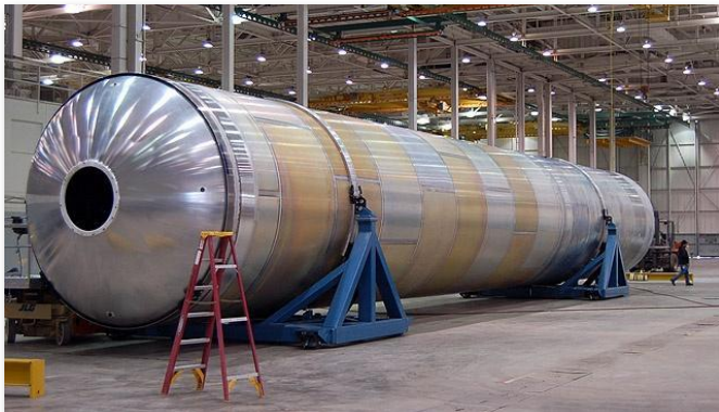
Falcon 9 first stage tank in production - Same diameter and length as a Boeing 737
