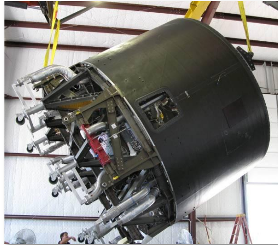
Thrust frame & plumbing for nine engines
