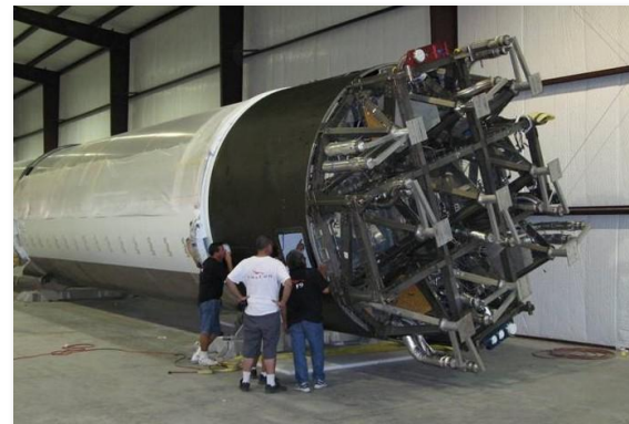
First stage mated with thrust frame
