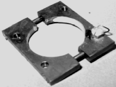
Figure 1. Copper heat intercepts, placed on the pulse-tube cooler between the first and second stages as indicated on figure 2.
