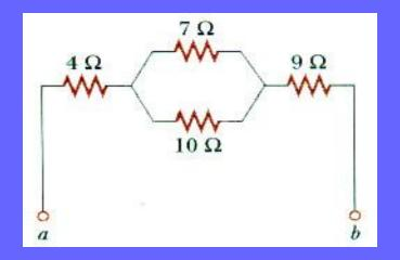
(b) If a potential difference of 34 V is applied between points a and b, calculate the current in **each** resistor.
