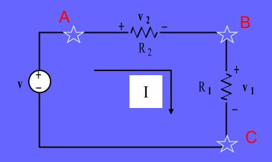
1. Because of the <u>charge conservation</u>, all charges going through the resistor  $R_2$  will also go through resistor  $R_1$ . Thus, currents in  $R_1$  and  $R_2$  are the same,
