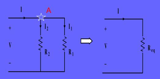
1. Since both  $R_1$  and  $R_2$  are connected to the same battery, potential differences across  $R_1$  and  $R_2$  are the same,
