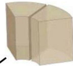
Tensile Failure Vertical (TFV)
