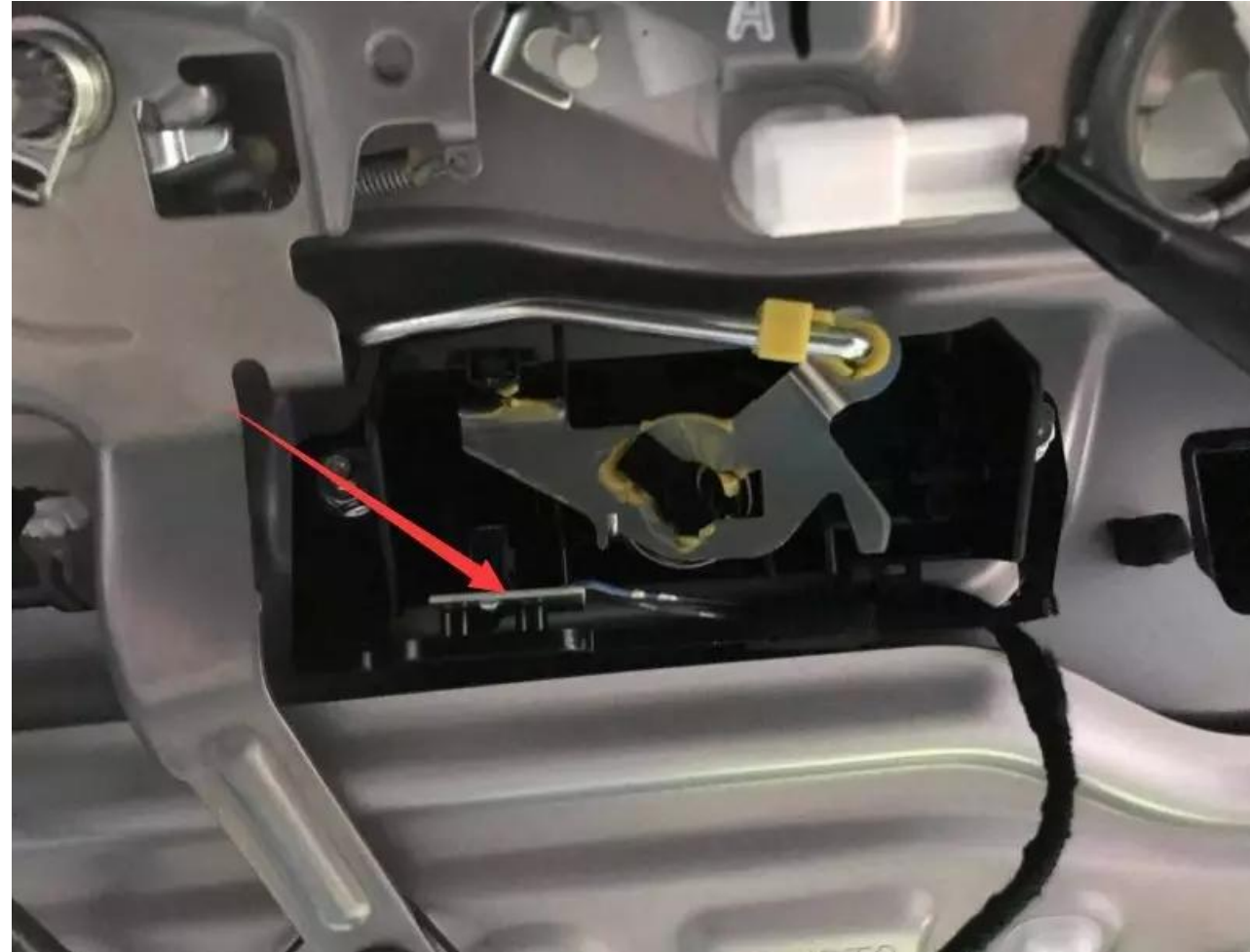
在后门此处焊接电动尾门专用把手开关，螺丝固定 Weld the electric tailgate handle switch here on the back door and fix it with screws
