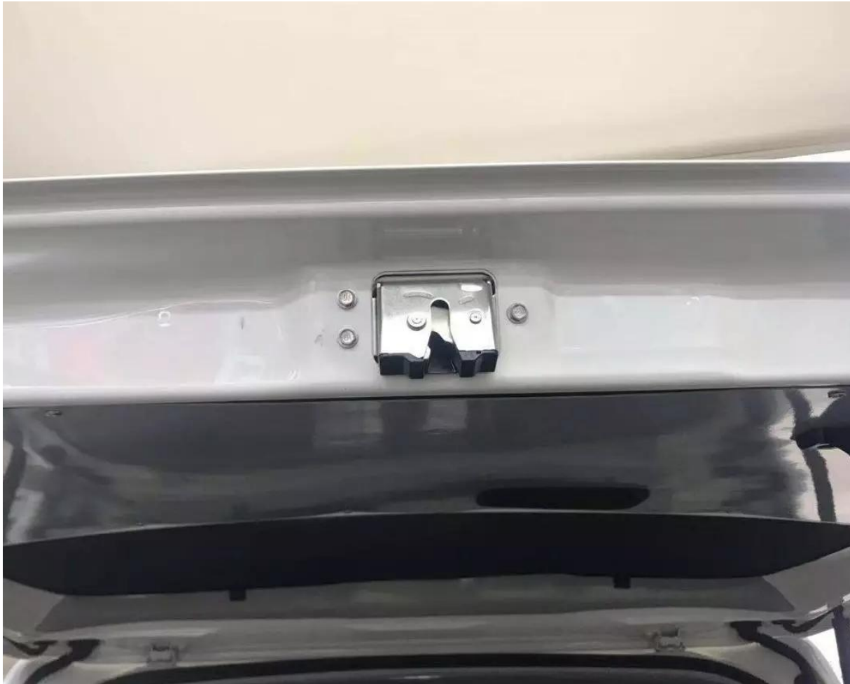
安装好钢丝后，把原车锁安装到原位置，用专用螺丝固定 After installing the wire, install the original car lock to the original position and fix it with special screws
