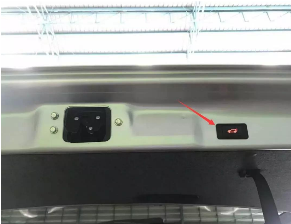
后门安装电动尾门关闭按钮 Install electric tailgate close button on back door
