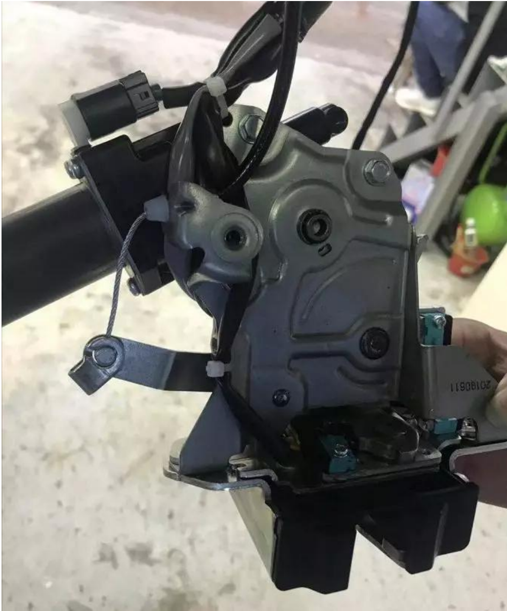
在原车锁上面安装电动尾门专用钢丝，钢丝卡入锁内 Install special wire for electric tailgate on the original car lock, and the wire locks into the lock
