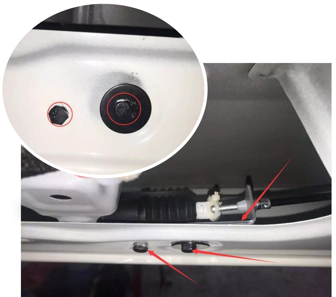
另一边在原车孔位固定执行器支架用螺丝固定 The other side fixes the actuator bracket in the original car hole with screws
