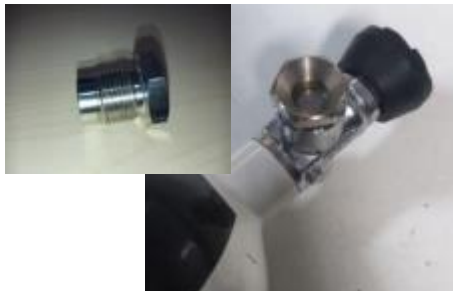
SCBA air cylinder during sudden release of air - projectile propelled through building
