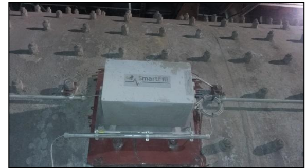
KIMA SmartFill "On Mill Unit" on Cement Mill no 3
