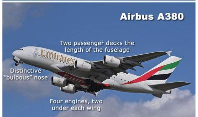
The A380 handles 600 people, with the right interior configuration. The A380 can handle all of their luggage, plus a fair amount of cargo. Having 4 engines, it has redundancy if there is an in-flight emergency.
