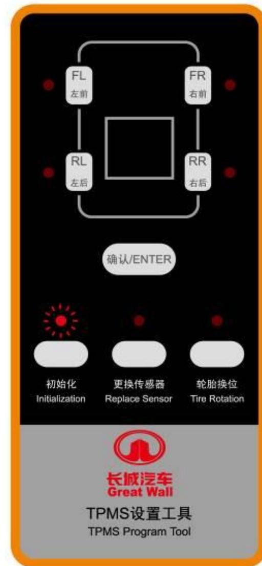
1.2 put TPMS program tool close to tyre valve nib within 50 cm to set sensor to be registered, press down corresponding tyre position button on program tool like “FL”, “FR”, then tyre position lamp will flash which means it’s waiting for signal from sensor as showed by right figure.
