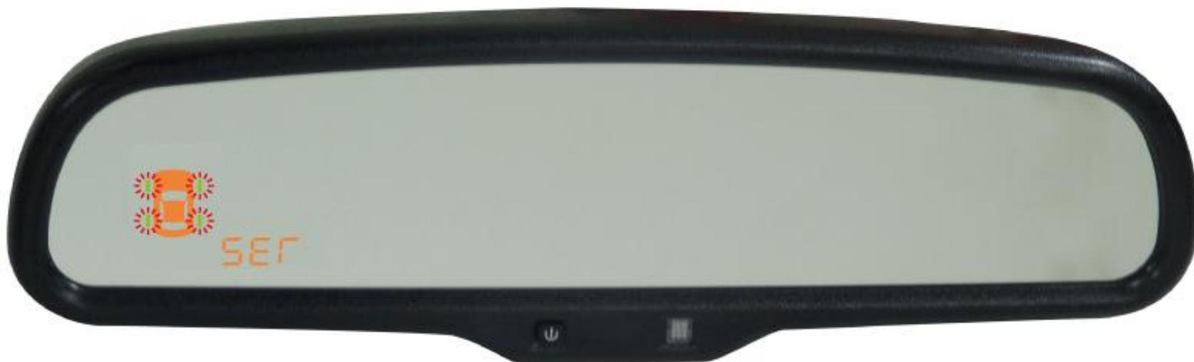
1.7 press “SET” button in the rear mirror with 30s as confirmation, then enter tyre pressure status display in circle, each interface will be shown for 3s as below figure.
