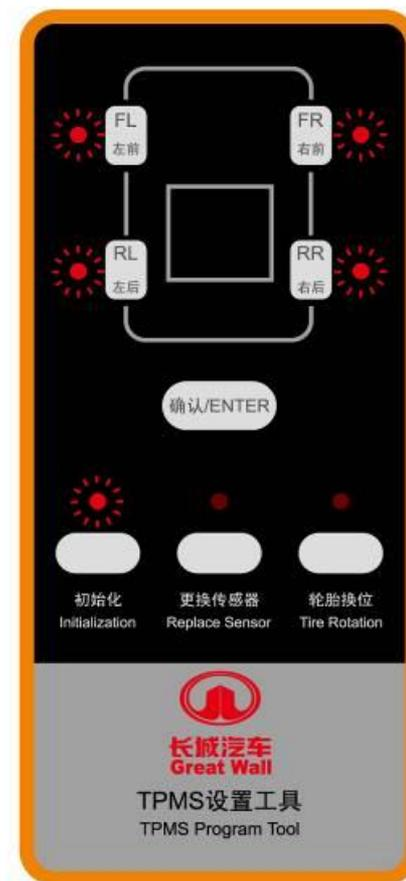
1.5 after 4 tyre indicating lamps light on, put TPMS program tool close to the receiver locating under driver seat (below figure) within 50cm, press down “ENTER” button, then all 4 tyre position lamp will flash in circle that sending out signals from registered sensor to receiver for saving.
