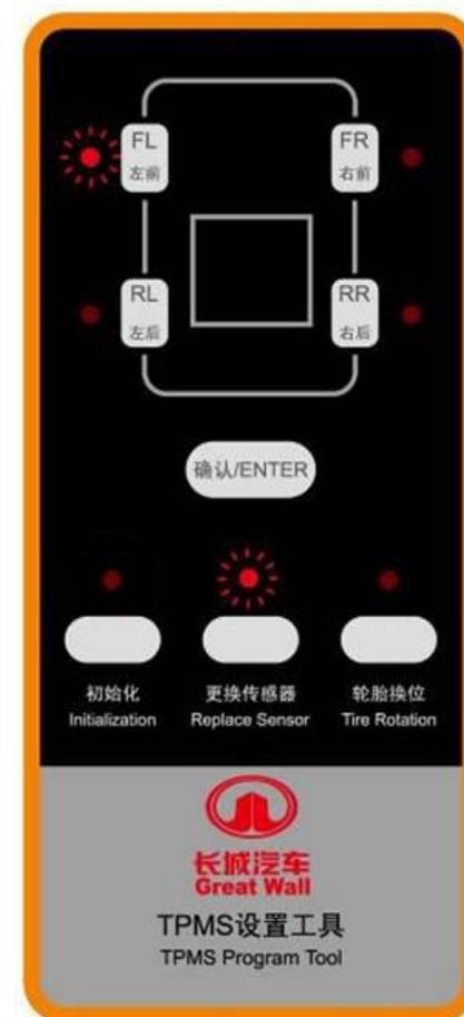
2.4 put TPMS program tool close to the receiver locating under driver seat within 50cm, press down “ENTER” button, then all 4 tyre position lamps will flash in sequence that sending out ID signals from sensor to be replaced to receiver for saving, after that there will be “ SET” displayed on rear mirror which means operation ok.
