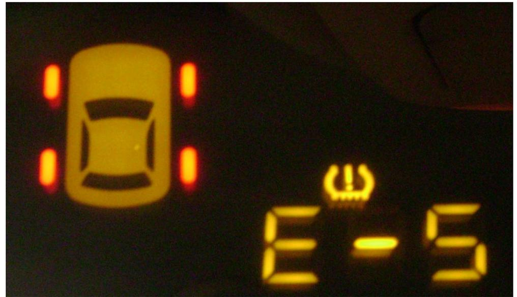
All 4 tyre indicators show red color and flash for 5s (0.5S off, 0.5S on), buzzer warns 5 times (sound 0.5S, silence 0.5S) tyre pressure warning sign ” and
