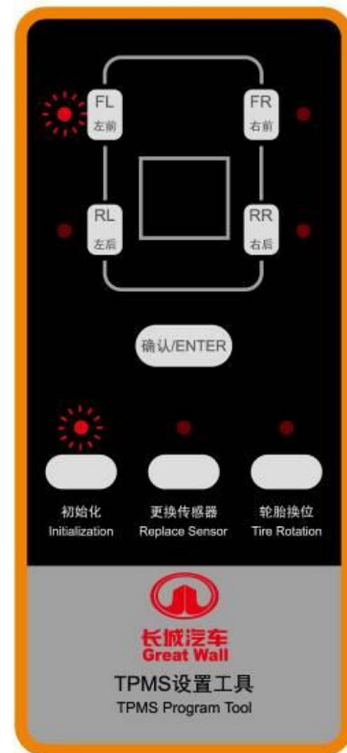
1.3 then register the other tyre position, of course, the lamps will keep on after register.
