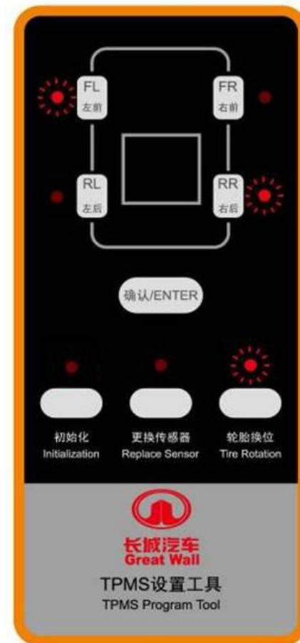
3.3 After selecting tyres to be exchanged each other, put TPMS program tool close to the receiver locating under driver seat within 50cm, press down “ENTER” button, then all 4 tyre position lamps will flash in sequence that sending out ID signals from sensor to be replaced to receiver for saving,
