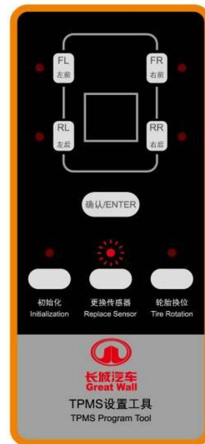
2.3 put TPMS program tool close to tyre valve nib within 50 cm, then press down corresponding tyre position button on program tool like “FL”, “FR”, then tyre position lamp will flash which means it’s waiting for signal from sensor, tyre position lamp will keep on as showed by right figure.
