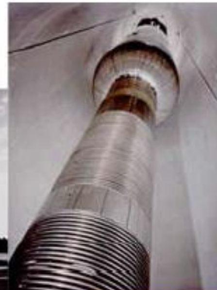
One of the two (face-to-face) stages of the 15 MV Tandem-Van de Graaff at BNL. Can accelerate 40 different types of ions.
