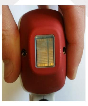
Shake the tip until it can be removed completely
