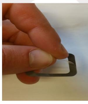
Remove the mat film covering the heat conductive
