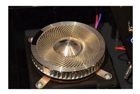
CoolChip has combined the heat sink and fan for added efficiency.
