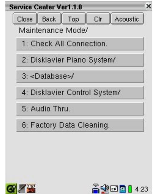
Press and hold keys [D], [M], and [P] in sequence within a second.
