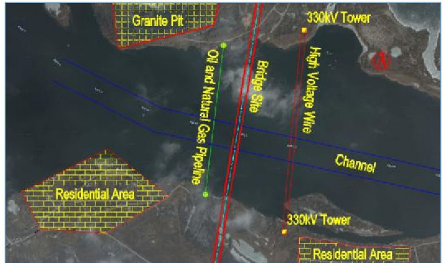
Bridge Position over Dnieper River
