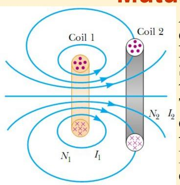
A cross-sectional view of two adjacent coils. The current  $I_1$  in coil 1, which has  $N_1$  turns, creates a magnetic field. Some of the magnetic field lines pass through coil 2, which has  $N_2$  turns. The magnetic flux caused by the current in coil 1 and passing through coil 2 is represented by  $F_{12}$ . The mutual inductance  $M_{12}$  of coil 2 with respect to coil 1 is:
