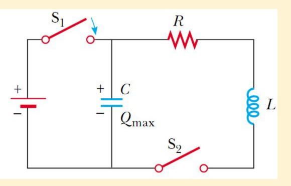
A series RLC circuit. Switch S₁ is closed and the capacitor is charged. S<sub>1</sub> is then opened and, at t = 0, switch S<sub>2</sub> is closed.
