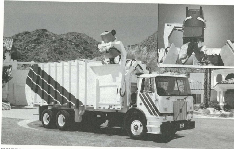
FIGURE 7.2 Typical example of mechanized collection vehicle with mechanical articulated pickup mechanism used for the collection of domestic source separated and comingled waste placed in a dual compartment container (see insert) (courtesy Heil Environmental Industries, Ltd.). The large containers equipped with wheels are brought to the curb by the homeowner. In some locations, helpers are used to bring the loaded containers to the curb, and the homeowner is responsible for returning the container to its storage location.
