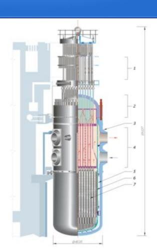
RBMK - High Power Channel-type Reactor
