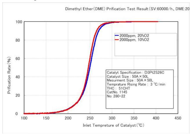
This data is just reference to be obtained from the result of the initial measurement by TKK. We don't design the catalyst using operation temperature in less than 100% of purification rate, because the catalyst lose purification the organic matter soon when the catalyst deteriorates during the operation. We recommend operation temperature is 300 C in your case.
