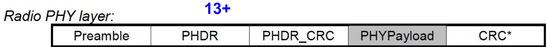
Figure 5: Radio PHY structure (CRC* is only available on uplink messages)
