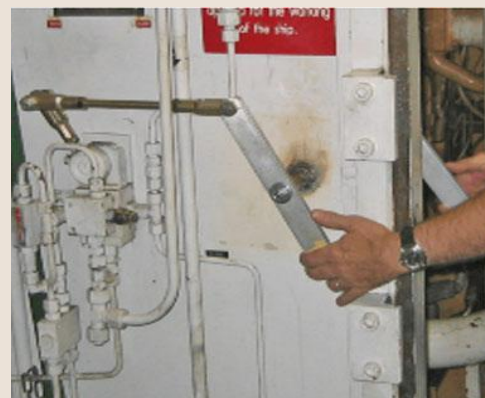
Water/Weather-tight doors not closing properly
