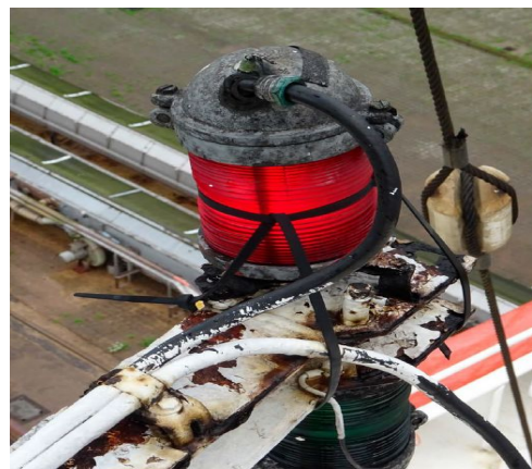
Signal lights not properly secured
