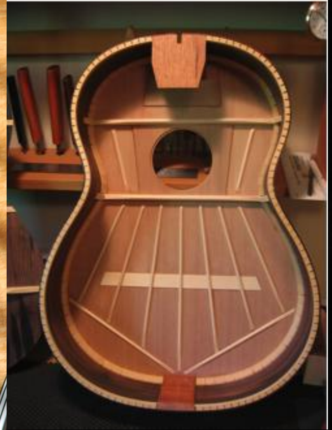
"fan" top bracing pattern
