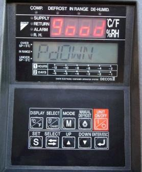
Press the  $\mathbf{M}$  key twice to select the pump down mode, then, the LCD indicates "**PdOWN**". Select "**on**" by using  $\Delta$  key or  $\nabla$  key.
