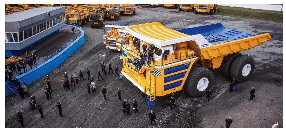
The monster truck has a diesel-electric transmission system. Two 16-cylinder diesel engines drive generators which produce electricity to power four electric motors – compare that to the four or six-cylinder engine that powers your average family car.
