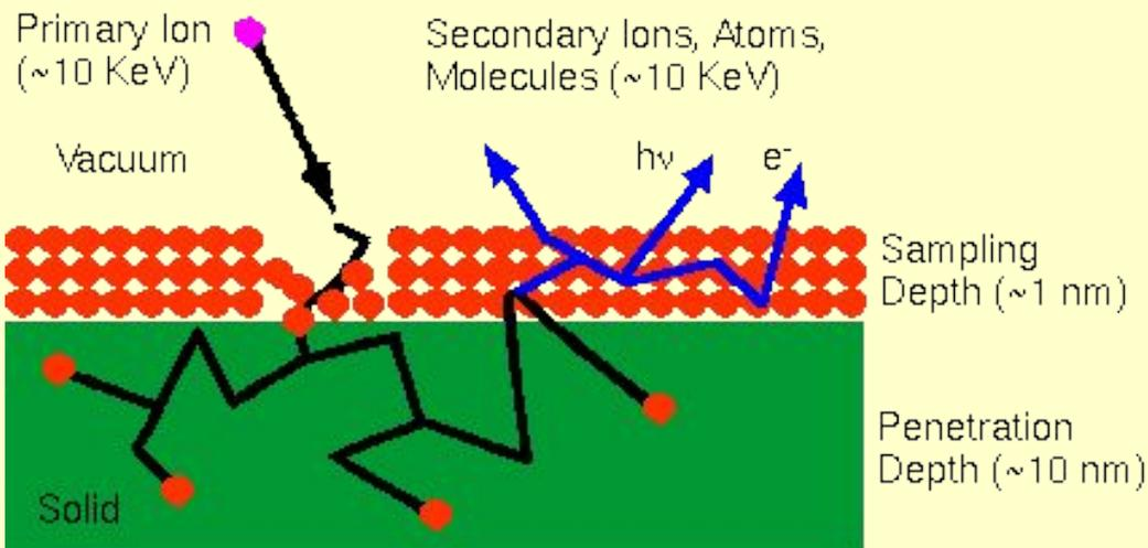
Effects of sputtering on the surface of the exposed material
