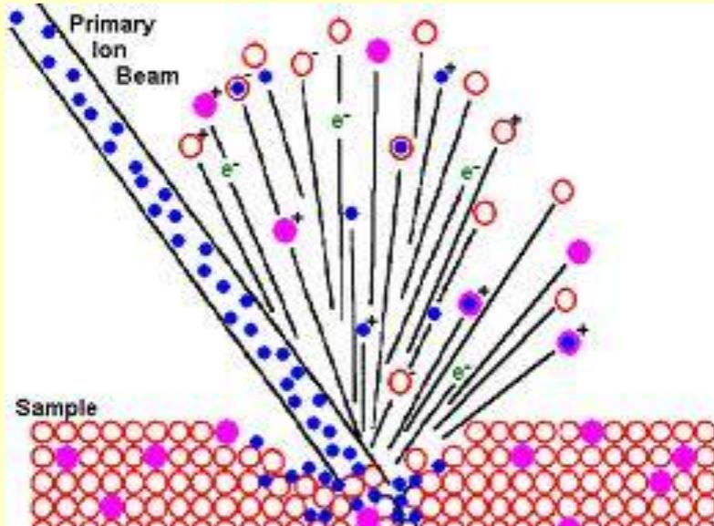
Sputtering (in the case of an intense ion beam)
