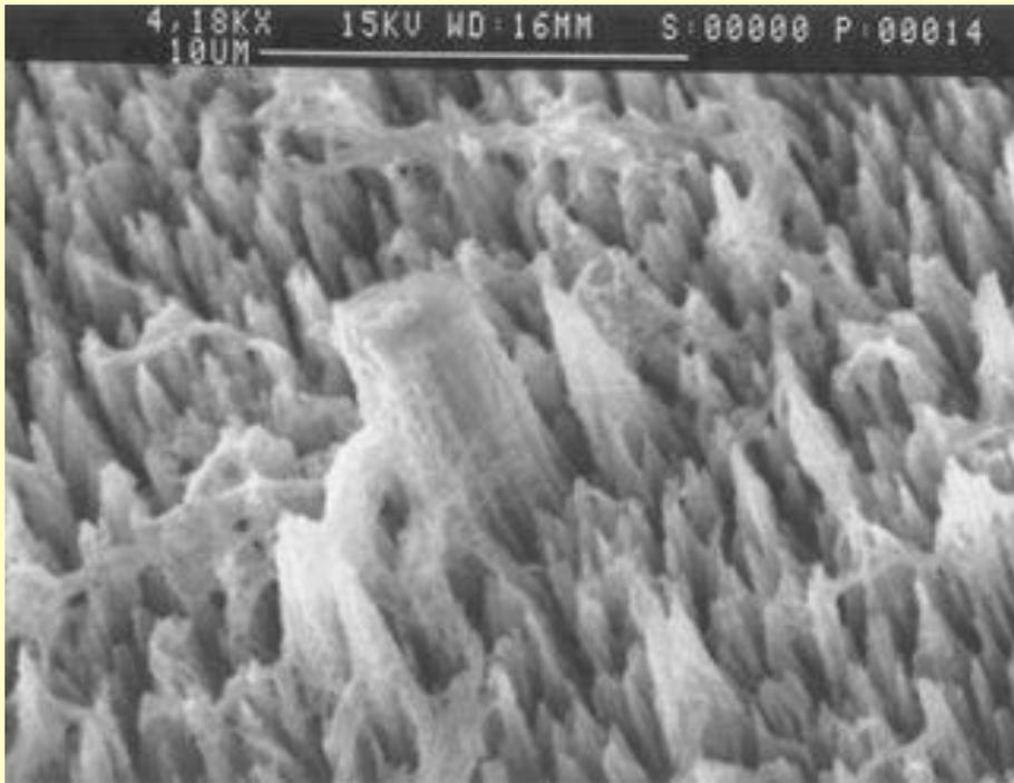
The surfaces exposed to AO erosion change substantially its surface roughness, and with it its thermal and optical properties
