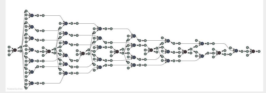
Bigger nodes represent microkernel calls performed by the computational cores, while smaller ones represent tile transfers between the main storage and LS.
