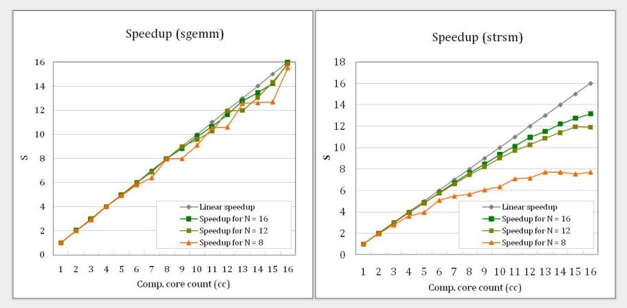
Scales almost linearly up to 16 cores of a synthetic multicore processor (Matrix size =  $N \cdot NB$ ).
