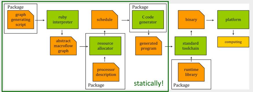
Our approach moves "decision-making" to compile-time, reducing the overhead level. It becomes possible, because, the computational process does not depend on particular data values.
