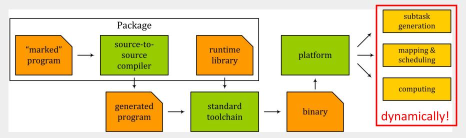
Existing toolchains (Cilk, StarS) make scheduling decisions at runtime. The runtime manages tasks (tile processing), distribute the workload, try to do its best in memory reuse, etc.
