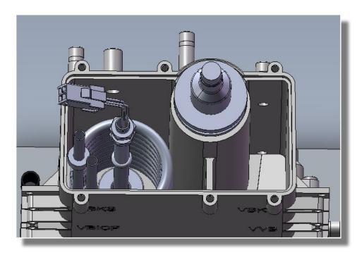
Components in the Upline Tank •Heat exchanger •Float Switch •Heater rod
