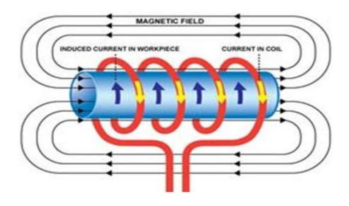
An inductor is often referred to as AC resistor. It resists the changes in the current and stores energy in the form of the magnetic field. These are simple in construction, consisting of the coils of copper wire wounded on a core. This core might be magnetic or air.
