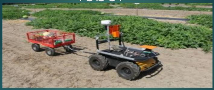
The cotton harvester robot was successfully assembled and tested on a field within the first three months of its development.
