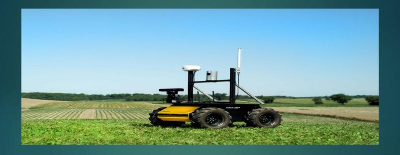
Since robots do not need a human driver, there is no need to maximize the efficiency of the driver, so the machines can be smaller and lighter, thus producing less soil compaction.
