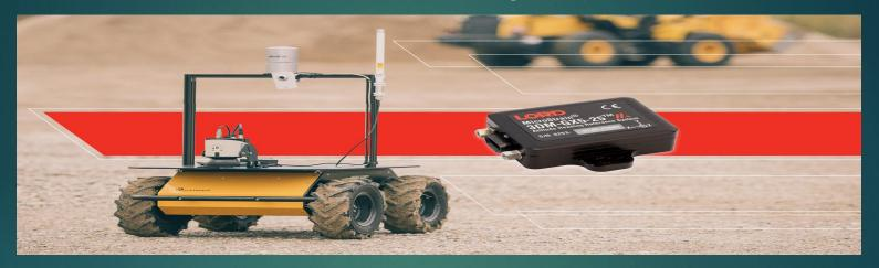
UGVs are powered by 24 V batteries and have a 5 V, 12 V and 24 V power distribution on the device. Depending on the payload, these vehicles can travel at a speed of about 2 mph for 2–3 hours before recharging is required.
