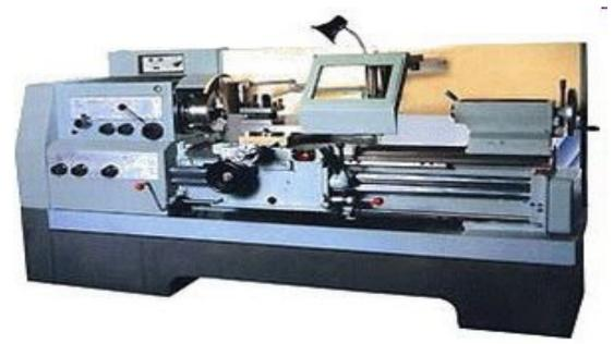
The saddle consists of a casting designed to carry the tool post slide or slides, and is fitted to the ways of the bed so that it may slide along it without lateral movement. The front of this casting called the apron, carries. The cross slide is mounted on the top of the saddle and must be at right angles to the bed.
