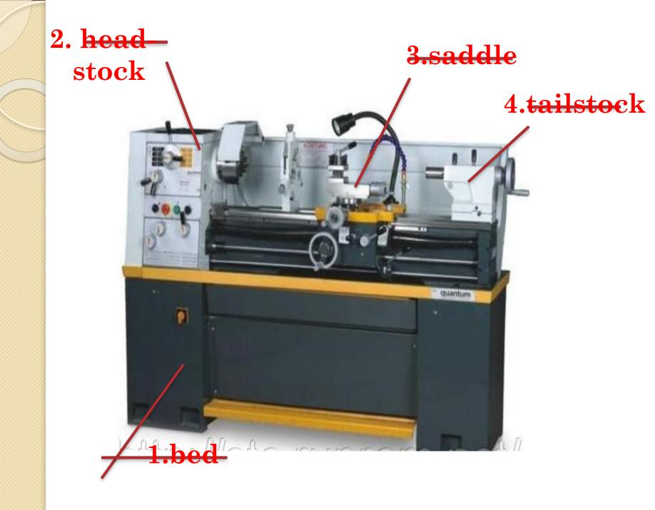
**The bed** – The main casting of the lathe is called the bed, and usually consists of a good quality grey iron casting of rigid design. It is provided with accurately machined ways, on which slides the saddle and the tailstock, and on which the headstock is located and bolted.
