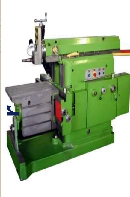
A shaper is a machine that surfaces by successive forms reciprocating cuts of a tool over the work. The work is stationary with reference to the tool but moves laterally in small steps so that the successive cuts be can Although most of the made. work performed on shapers consists of plane horizontal surfaces, it is also possible to finish vertical and angular surfaces, and, with the proper tools and accessories, even
