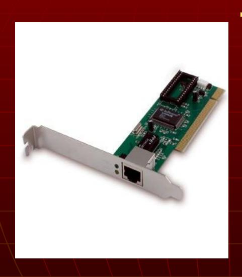
A network card is a card, a device, installed on the motherboard or integrated into it. A network card is used to connect a computer to other computers over a local network or to connect to the Internet.
