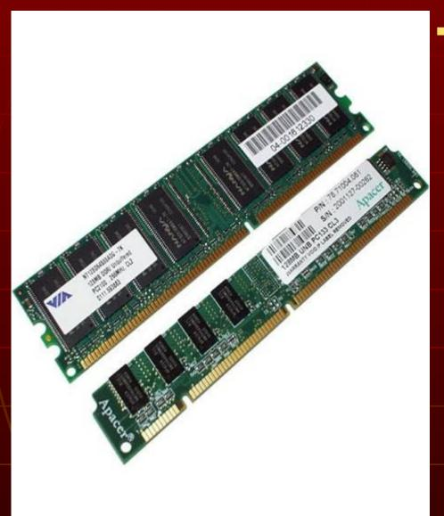
**RAM** - memory for temporary storage of data in the computer, is used only when the computer is running. The speed of the computer depends on the amount and the speed of RAM.
