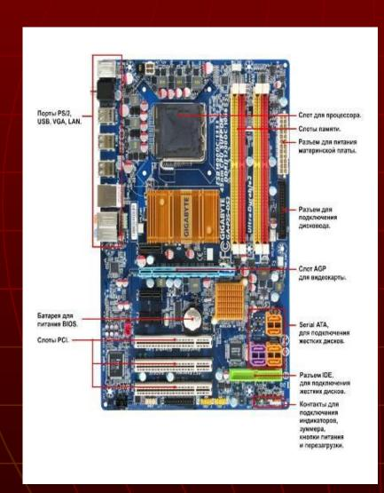
The motherboard is the main part of the system unit to which all devices of the system unit are connected. Through the motherboard there is a communication between the devices of the system unit, information exchange and power supply. The faster the bus (communication channels of devices) of the motherboard, the faster the communication of devices among themselves, the faster works the computer.
