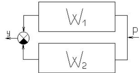
$$W_{эус} = \frac{y}{P} = \frac{\varepsilon_1}{k_1 (T_1^2 p^2 + T_2 p + 1)} - \frac{\varepsilon_2}{k_2 (T_1'^2 p^2 + T_2' p + 1)}$$
