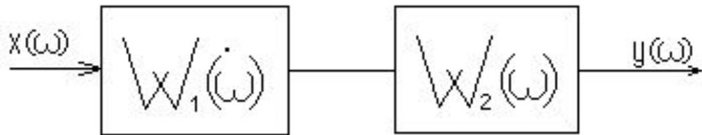
$$W_{\Sigma} = \frac{y(\omega)}{x(\omega)} = W_1(\omega) \cdot W_2(\omega)$$
