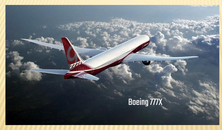
The Boeing 777X is the latest series of the long-range from **Boeing Commercial** Airplanes. The 777X will feature new GE9X engines, new composite wings with folding wingtips, greater cabin width and seating capacity, and technologies from the Boeing
