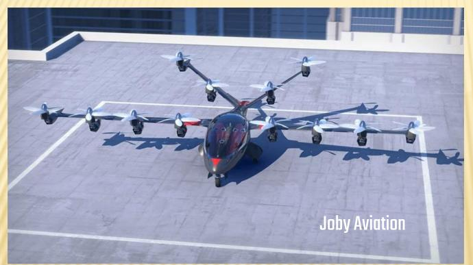
When cruising speeds are reached, these propellers will fold and the aircraft will fly thanks to four more propellers located behind the wings and tail.
