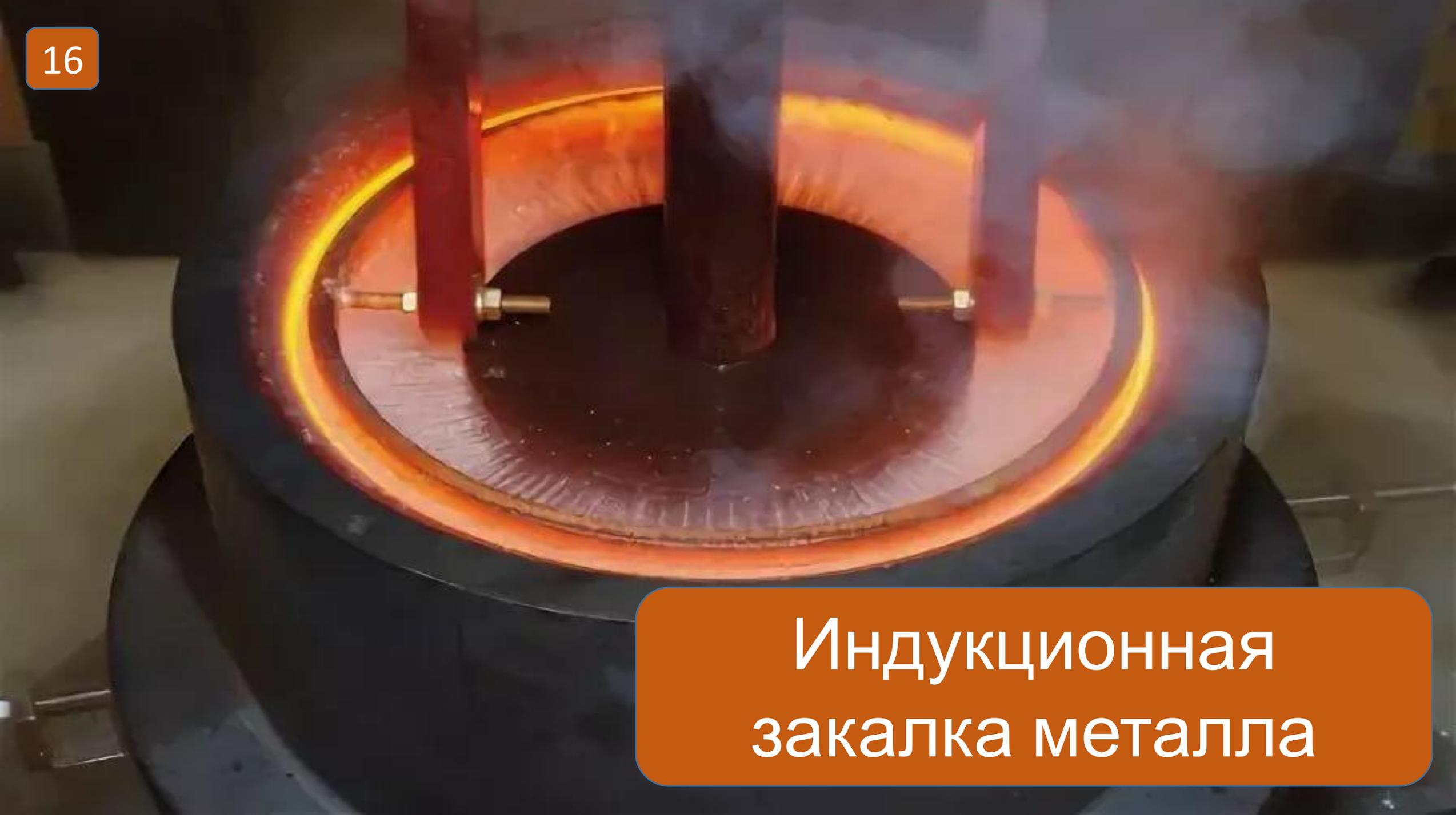
A close-up photograph of an industrial induction quenching process. A large, dark metal workpiece is being heated by a glowing orange-red induction coil. The workpiece is mounted on a central shaft and is surrounded by a liquid quenching medium. The background is dark and industrial.
