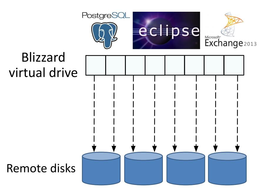
The naïve approach for implementing virtual disks does not maximize spindle parallelism for POSIX/Win32 applications which frequently issue fsync() operations to maintain consistency.
