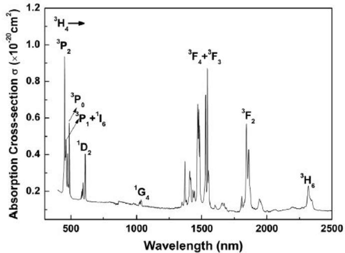
2 Room temperature absorption spectrum of Pr:YAG crystal
