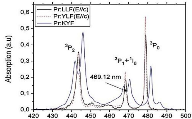
Fig. 1. Room temperature absorption spectra of Pr:LLF, Pr:YLF and Pr:KYF in the blue spectral range.
