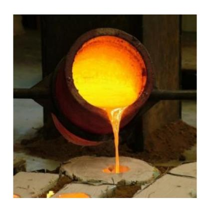
First, wooden templates are made, and sand forms are based on them. After that, the molten metal is poured into the sand mold, which gradually solidifies. When the resulting cast is removed, the mold is destroyed.
