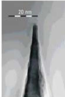
SEM image of Ultrasharp silicon tip
