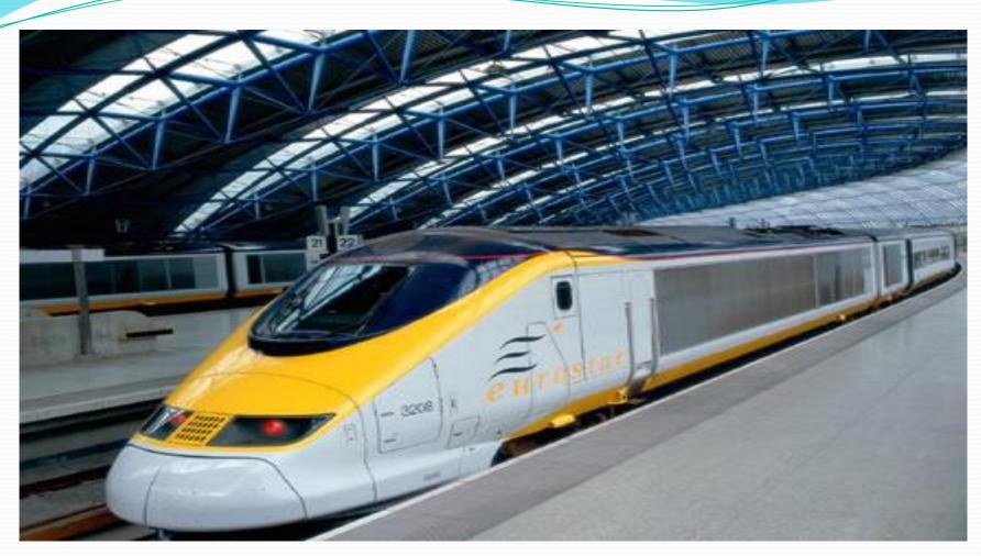
High-speed movement (up to 250 km/h) in trains, consisting of wagons with tilt body, is made on enhancements to existing lines. Fast trains on the route London - York developing speed 180,2 km/h; train «Eurostar», linking London with the continental Europe,-209 km/h (restricted when passing the tunnel under the English channel).
