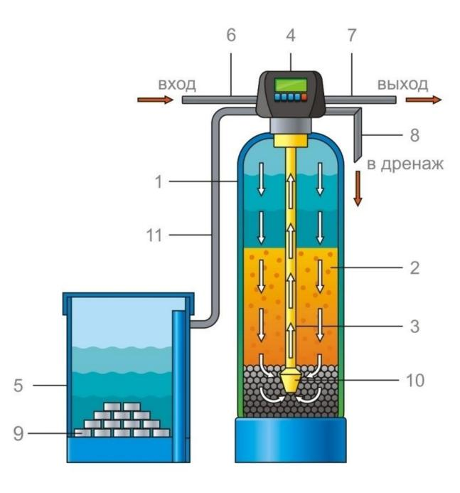
filter housing (1), filtering bed (2), automatic control valve (4), inlet pipe (6), outflow pipeline for purified water (7), drainage pipe (8) and drainage-distributing device (3; 10). preparation tank for regeneration of filtering bed (5). tableted salt (9).
