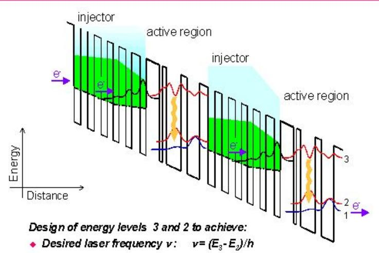
Light amplification: level 3 full of electrons; level 2 empty of electrons
