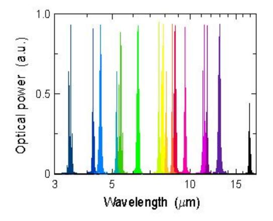
QC lasers cover entire mid-infrared wavelength range (3.4 - 17 µm) by tailoring layer thicknesses of the same material
