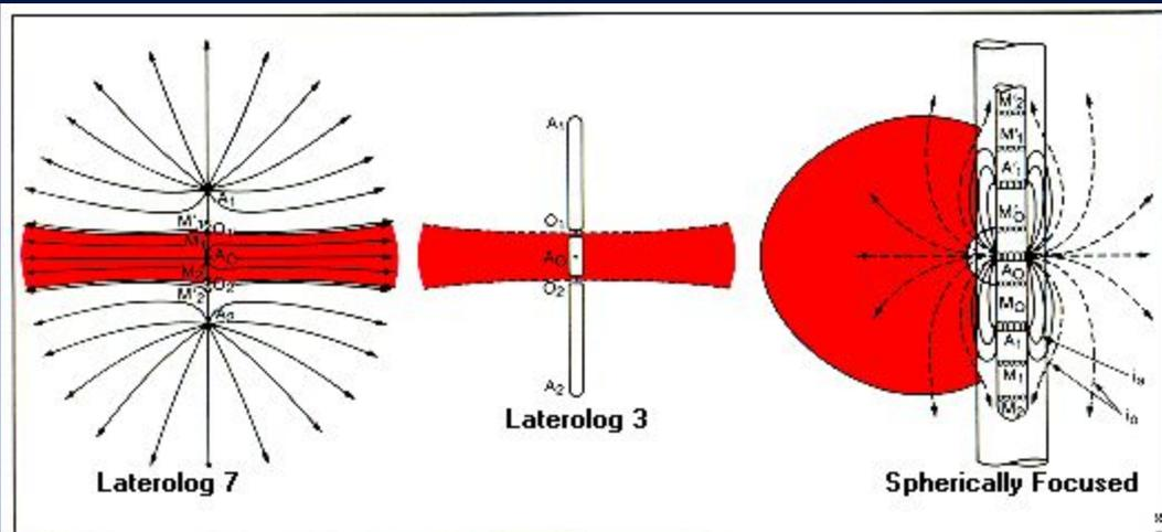
Fig. 7-10—Schematics of focusing electrode devices.
