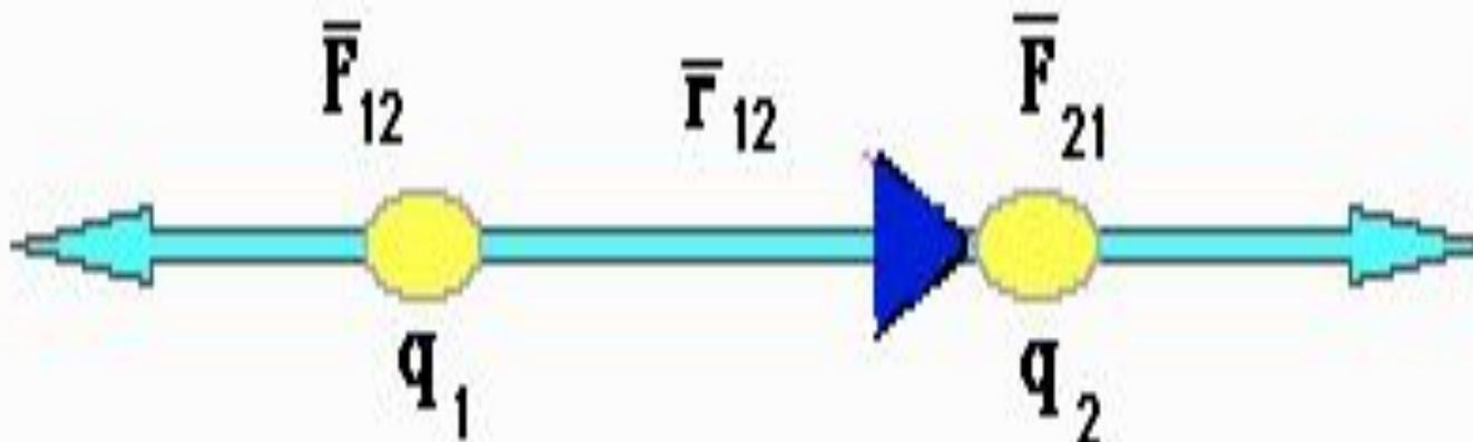
$$\bar{F}_{21} = k \frac{q_1 q_2}{\mathcal{E} r_{12}^2} \cdot \frac{\bar{r}_{12}}{r_{12}}$$
