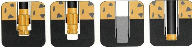
1 When drilling starts, the ODEX reamer swings out and reams the pilot-hole wide enough for the casing tube to slide down behind the drill bit assembly.
